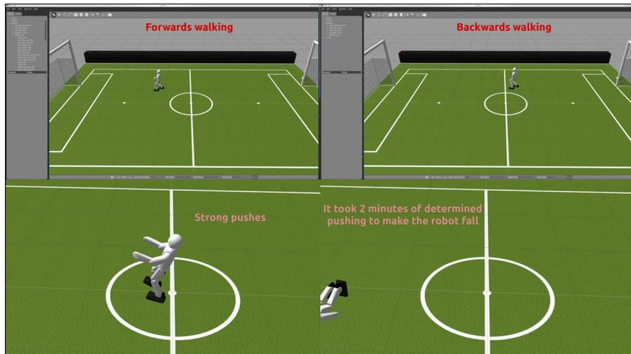
Video 11.4: Summary video of the first walking and balance tests that were performed (in simulation) to evaluate the effectiveness of the tilt phase controller. The simulated igus Humanoid Open Platform withstood two minutes of strong pushes before eventually falling. [https://youtu.be/A\\_HQQfCRhDE](https://youtu.be/A_HQQfCRhDE)
