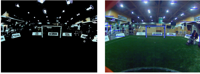
(a) White color segmented image in which pixels that are not considered to be white have been painted black. (b) Result after merging all extracted horizontal and vertical white line segments (annotated in blue).
