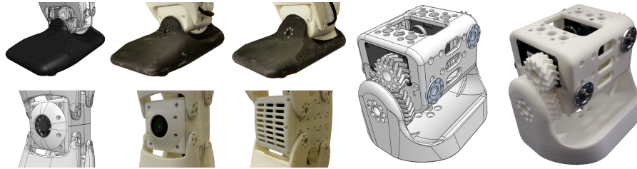
Fig. 2. Comparison of various hardware design features. Left: foot and back side of the knee: OP2X(CAD), OP2X, OP2. Right: Finished hip joint along with the CAD model showing the 3D-printed gears on the NimbRo-OP2X.
