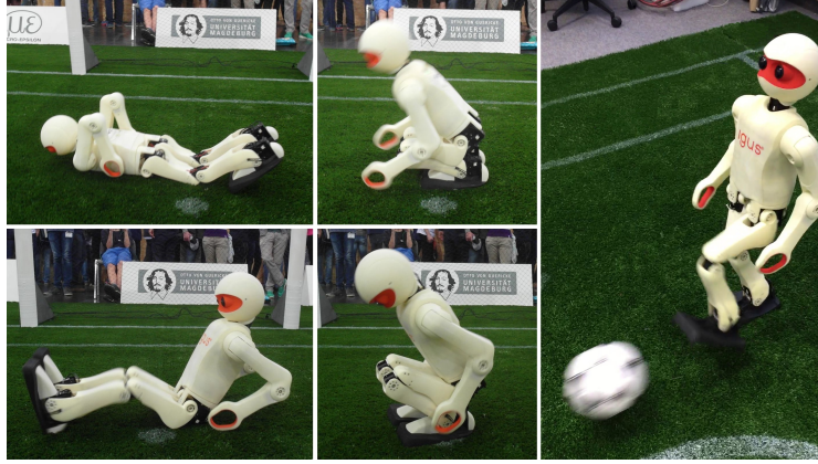
Fig. 6. Dynamic get-up motions of the igus Humanoid Open Platform, from the prone (top row) and supine (bottom row) lying positions, and a still image of the kick motion.
