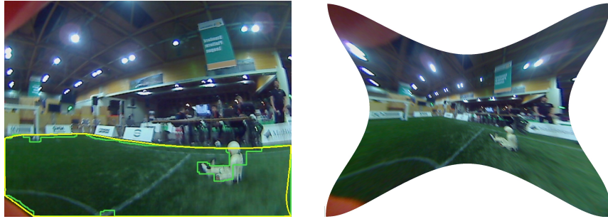
Fig. 3. Left: An image captured by the robot with annotation of the detected field boundary. Right: The effect of applying the undistortion model on the left image.
