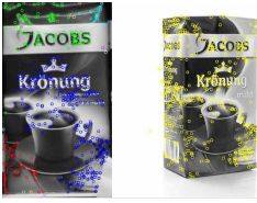
Fig. 4. Object recognition using vocabulary trees and SIFT features. Left: test image, right: matching template from www.germandeli.com database.
