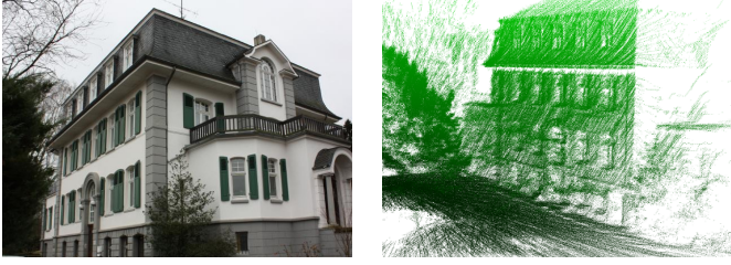
Fig. 6. Resulting map of the Frankenforst outdoor dataset obtained by the surfel registration (lowest MAP-MME).
