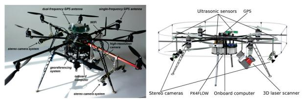
Figure 1: The two MAVs, as they are developed within the project. Left: IGGKopter. Right: AISKopter
