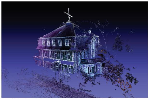
Figure 12: Georeferenced point cloud, extracted from images using a freely available software package for dense image matching (Furukawa, 2010).
