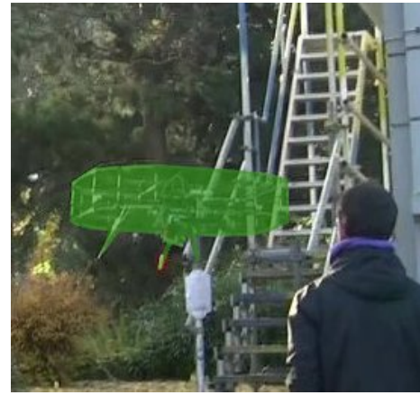
Fig. 9: Reactive collision avoidance can act as a safety layer between commands given by higher-lever planning layers or a human pilot. It can help to navigate the robot (green) in challenging situations.
