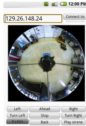
Figure 6. User interface of teleoperator software in the Android environment.
