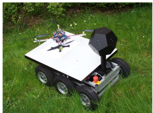
Figure 1. First conceptual chassis of the UGAV . The ground platform is built on a VolksBot RT6 which is equipped with a panoramic vision system (sphere cube with 11 cameras) and a landing platform for the quadrotor.
