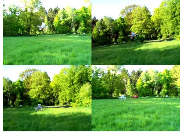
Figure 8. Most salient regions in four frames of the quadrotor flight. In more than 80% of the images is the quadrotor the most attentive object. When a red car drives through the scene the attention goes to it (bottom right) A video with all images can be found under http://www.volksbot.de/videos/vocus_copter-2008.avi .
