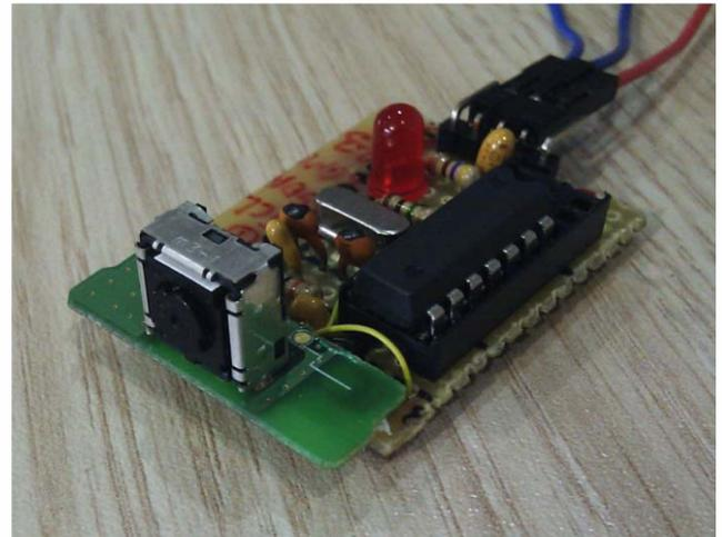
Fig. 1. The prototype of driver board for communicating with PixArt camera. The small camera in the left side of picture is the PixArt camera.
