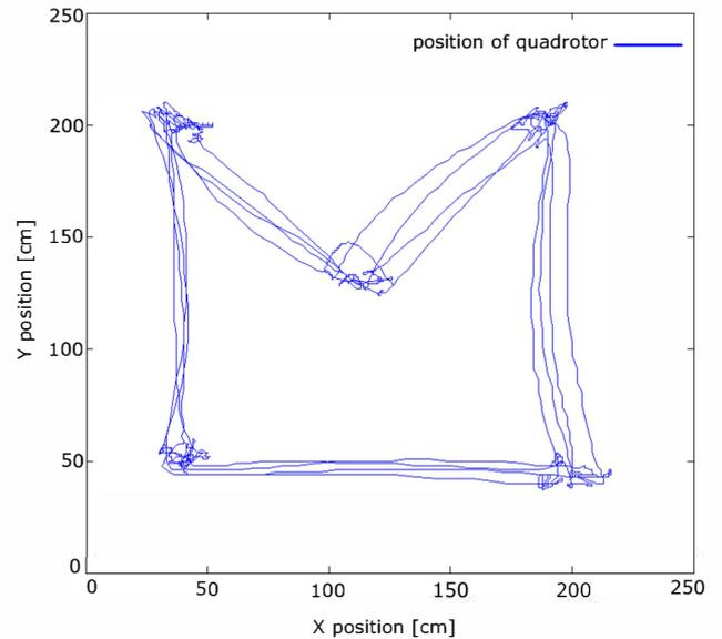
Fig. 8. Position regulation in a set of five different points.
