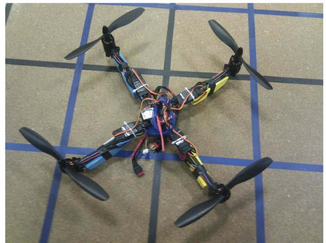
Fig. 2. Picture of our custom build quadrotor.
