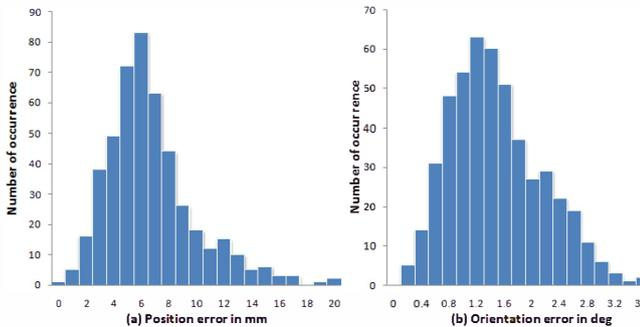
Fig. 6. Distributions of position and orientation errors measured in the  $2 \times 2 \times 1 [m^3]$  working space.
