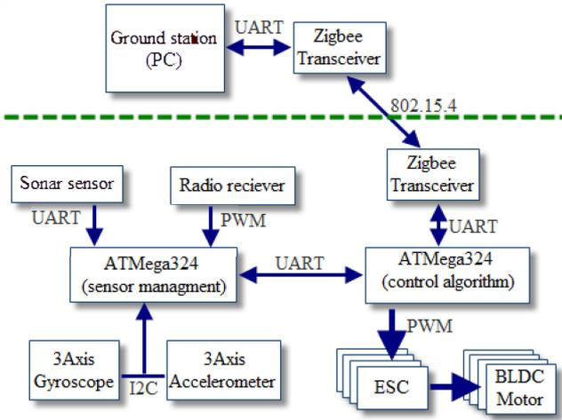
Fig. 3. System architecture of the quadrotor and ground station.
