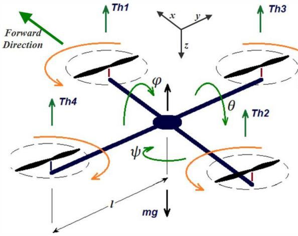
Fig. 5. The quadrotor schematic.
