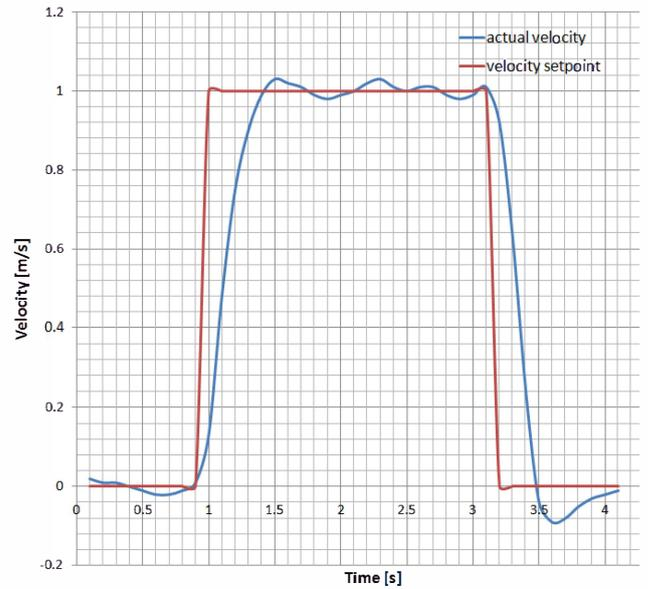
Fig. 7. System’s velocity response to a pulse input
