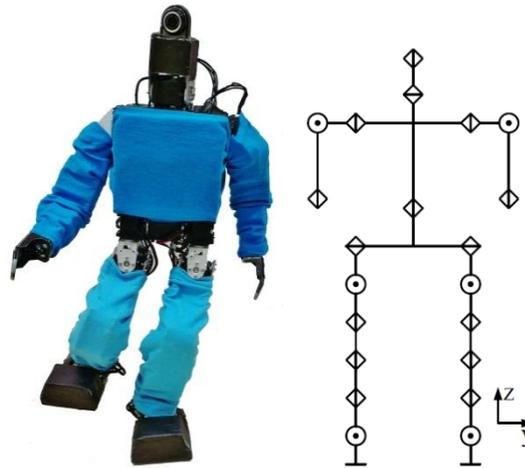
Figure 1. AUTMan “DROID2013” robot (left) and its kinematic
