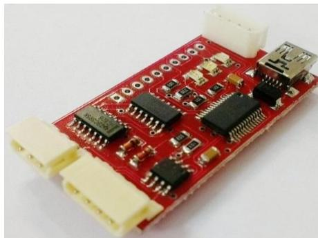
Figure 2. 9DOF IMU and RM-G146 sensor module
