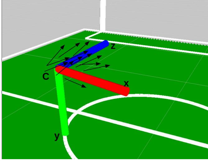
**Figure 4.19:** The  $(C, x, y, z)$  is the camera coordinate system, with z-axis pointing to the center of captured images. The origin of this coordinate is the estimated camera position. The black arrows are hypotheses generated around the current state.
