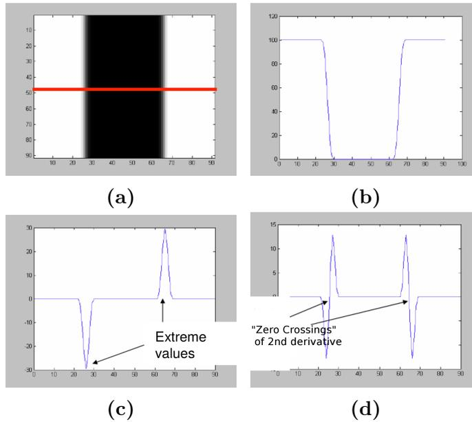
**Figure 3.6:** Line detectors. (a) A line with two vertical edges. (b) Intensity function (along horizontal scan line). Edges are regions with a high slope. (c) The first derivative of the intensity function. High slopes are found from the maximum /minimum of the first derivative. (d) High slopes are found from the zero crossings of the second derivative.
