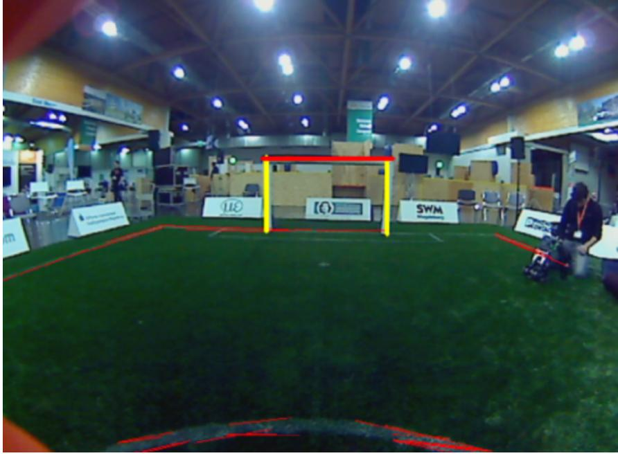
**Figure 2.1:** Output of the probabilistic Hough line detection on the extracted edges(Farazi, Allgeuer, and Behnke, 2015)
