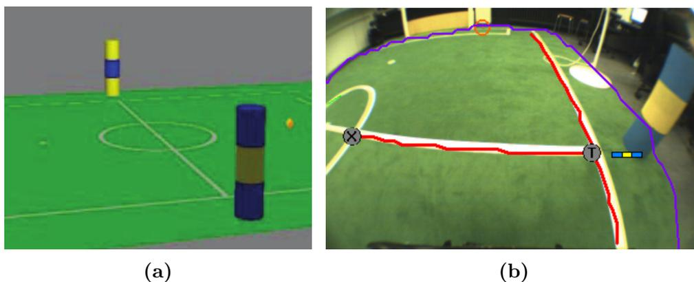
**Figure 2.3:** Field features: a) field landmark: poles; b) field crossings (Schulz and Behnke, 2012).
