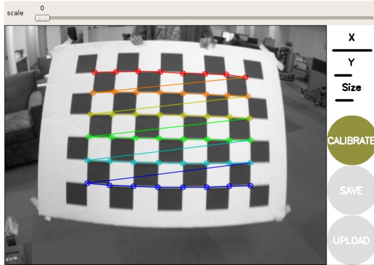
**Figure 3.2:** A calibration grid used for the estimation of the camera calibration matrix (Bradknox, 2015).
