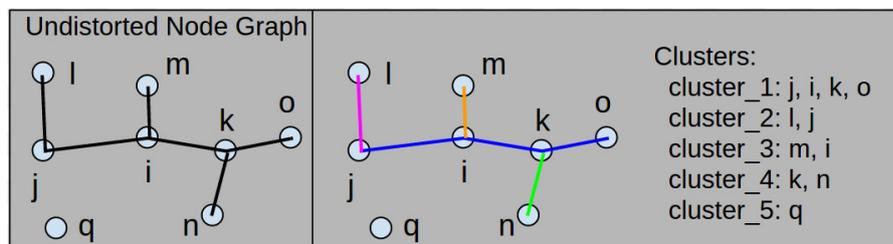
**Figure 1:** An example for extracting clusters from a node graph. Five clusters: four of which are in red, orange, blue, green respectively, and the fifth cluster contains a single node are extracted from the left node graph.
