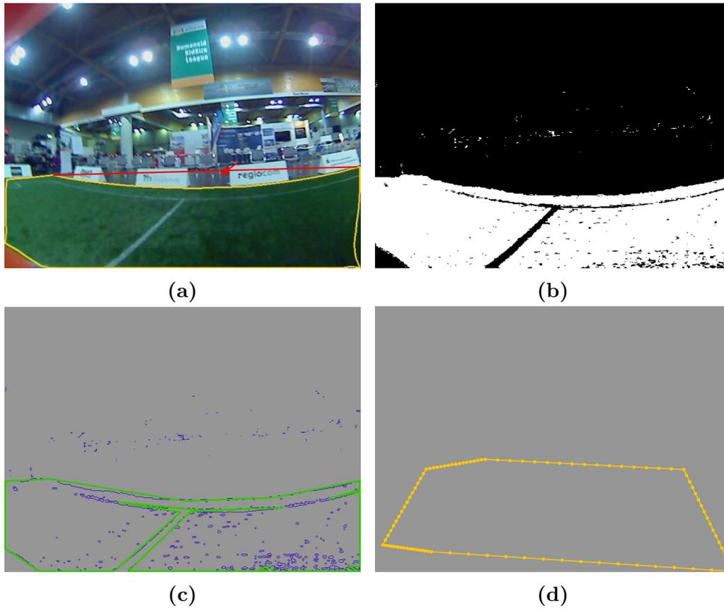
**Figure 4.2:** Field boundary detection. (a) Convex hull of the green regions in the image (yellow), and the unwanted area (red arrows). (b) Green binary image. (c) Contours based on segmentation. (d) Boundary points of the undistorted convex hull.
