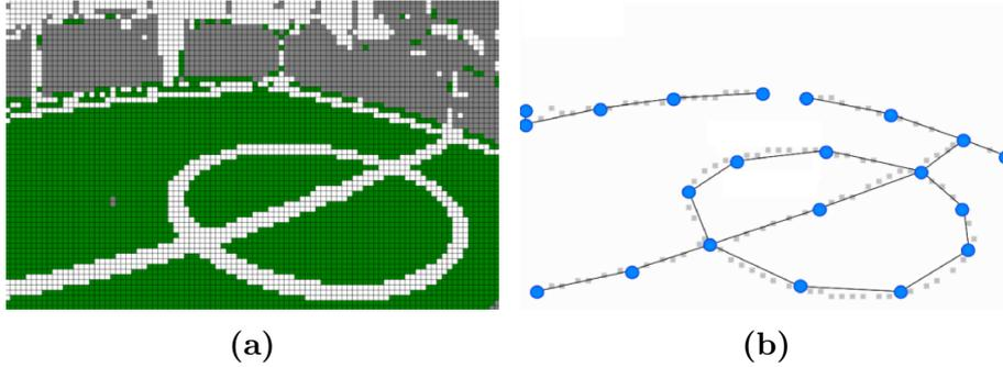
**Figure 2.2:** Node graph representation of field lines (a) subsampled image of pixels classified as “white” and “green”; (b) key node structure graph (Schulz and Behnke, 2012).
