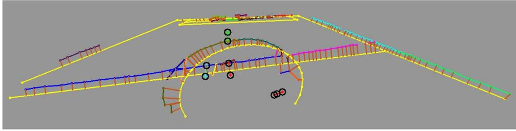
**Figure 4.17:** Data registration based on current estimated camera pose: the projected model is represented by yellow line segments; the observations are visualized using different colors for different clusters; each observed inlier node  $v_i$  is connected to its closest point  $c_i$  by a line segment in orange; nodes in black circles are identified as outliers.
