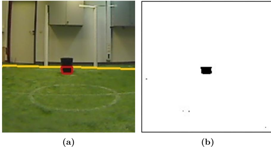
**Figure 4.4:** Obstacle detection. (a) Obstacle inside the green field (red). (b) Black binary image.
