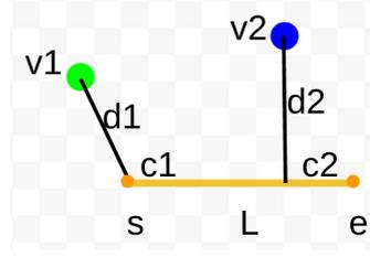
**Figure 4.16:** Examples of showing the distance of a node to a line segment: the closest point on line segment  $L$  to  $v1$  is  $c1 = s$ , so  $dist(v1, L) = \|v1 - c1\|_2$ ; while the closest point on line segment  $L$  to  $v2$  is the projected point  $c2$ , so  $dist(v2, L) = \|v2 - c2\|_2$ .
