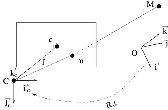
**Figure 3.1:** Ideal pinhole camera model describes the relationship between a 3D point  $M$  and its corresponding 2D projection  $m$  onto the image plane (Lepetit and Fua, 2005).
