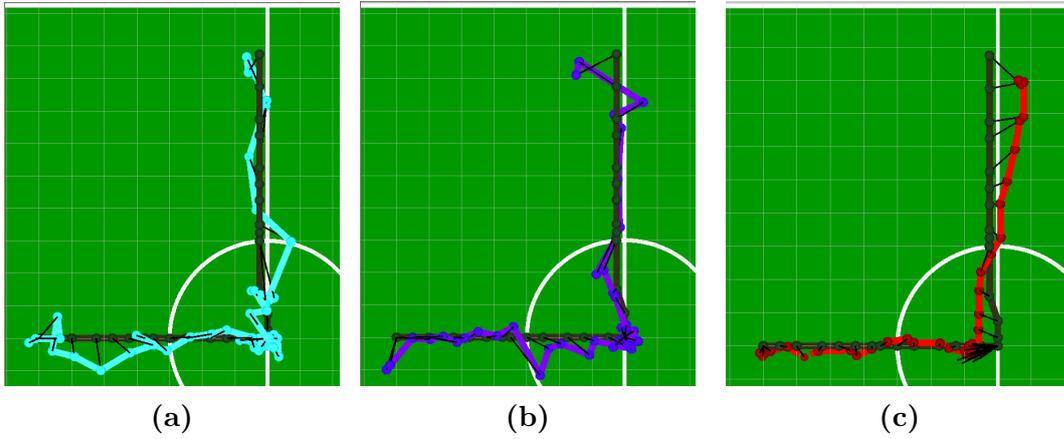
**Figure 5.5:** Evaluation on T9 test: (a) EPnP+RANSAC for pose optimization; (b) EPnP+RANSAC for pose optimization and Kalman filter for state fusion; (c) using Farazi's approach. The unit of grid is 20 cm \* 20 cm.
