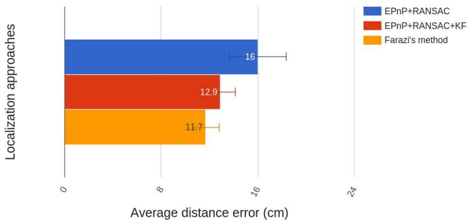
**Figure 5.6:** Average distance error of three types of localization approaches. The error bars in the figure indicates the standard deviations.
