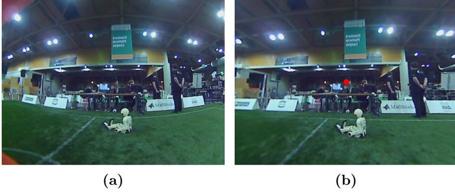
**Figure 3.4:** Undistorting an image. (a) Due to distortion effect, projections of straight lines are curved. (b) After undistortion, the projections of straight lines are straight.
