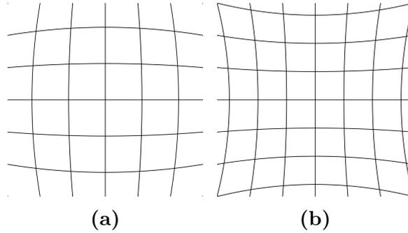
**Figure 3.3:** Two types of lens distortion: (a) barrel; (b) pincushion.
