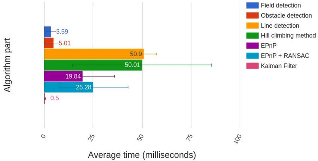
**Figure 5.2:** Execution time of each part of visual tracking system. The error bars in the figures indicate the standard deviations.
