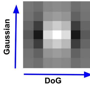
**Figure 4.6:** A 2D line filter for detecting vertical lines.
