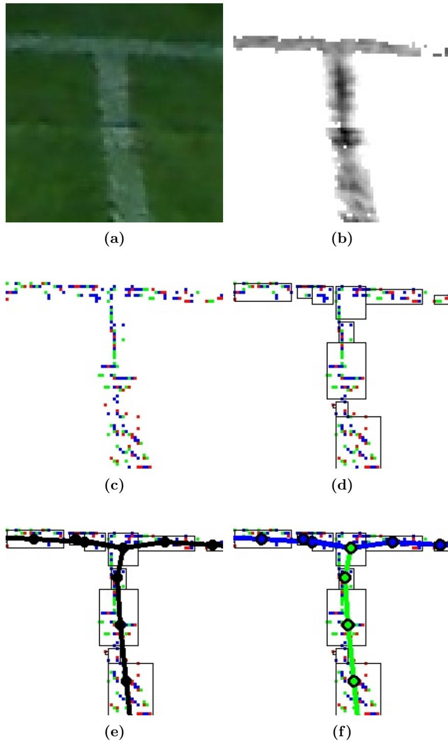
**Figure 4.11:** An example of field line detection process. (a)Input image. (b) The output brightness response image after applying line filters. (c) Three types of optimal values including: type 1 (red), type 2 (green) and type 3 (blue). (d) Bounding squares found from the optimal values. (e) A node graph constructed by connecting neighborhood squares. (f) Two clusters (in green and blue) extracted from node graph.
