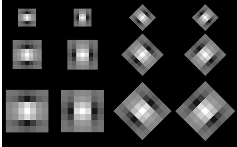
**Figure 4.7:** Four kernels used for detecting oriented line segments in three different sizes.
