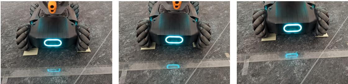
Figure 4.1: Precision test setup. We show three iterations of the test after the robot reached the target. The origin was marked with yellow papers directly under the front wheels.
