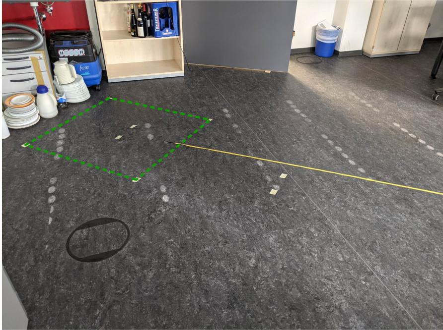
Figure 4.3: Calibration test setup. The calibration area of  $1\text{ m}^2$  is marked with green dashed line, the distance was measured with the yellow ruler.
