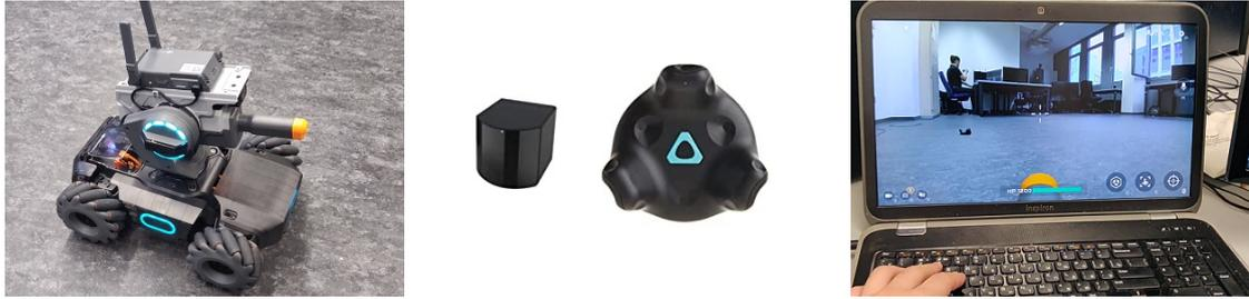
(a) DJI Robomaster S1. (b) Steam VR tracking system. (c) Windows machine with DJI controller.
