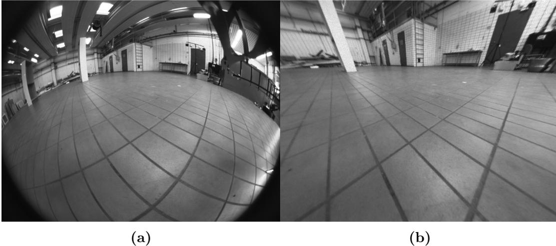
**Figure 4.5:** Stereo Rectification with TCC. Raw fish eye images (a) are rectified onto a plane with half the resolution (b).
