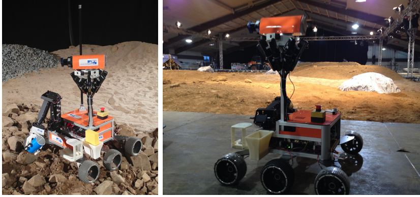
FIGURE 1.1: The Explorer robot platform developed by the University of Bonn pictured with the DLR Spacebot Cup arena.
