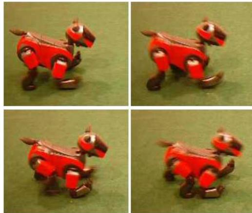
Figure 4.1: Aibo robot using the PWalk-style (Image from [41])
