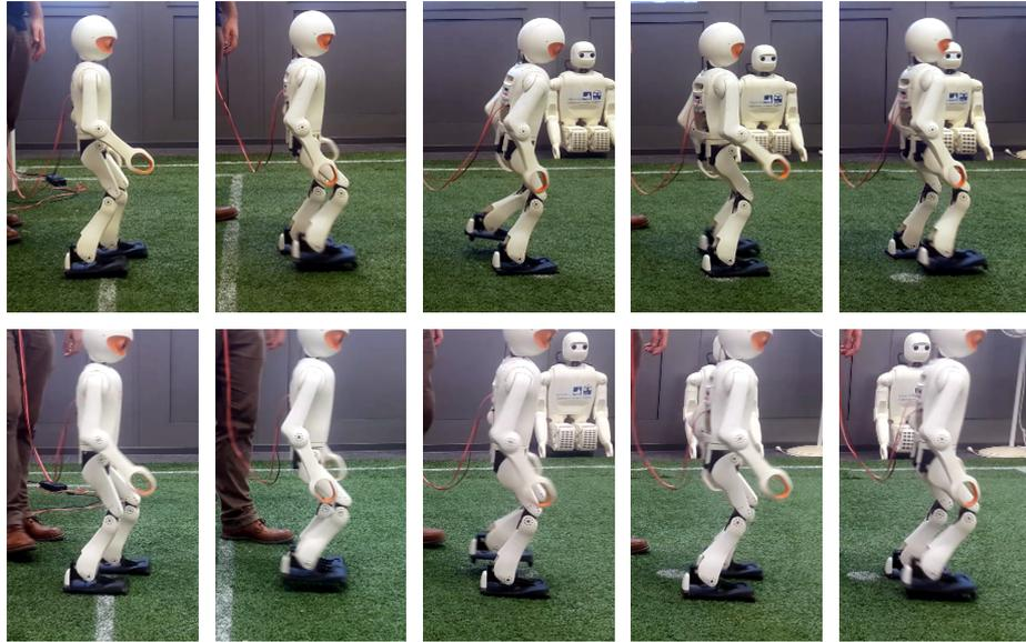
Figure 6.13: The igus<sup>®</sup> Humanoid Open Platform is performing gait evaluations. The top sequence shows the manually tuned gait, whereas at the bottom the resulting gait of the 4D optimized parameters is displayed. Qualitatively, it is possible to see that the magnitude of the robots tilt is smaller in the top sequence.
