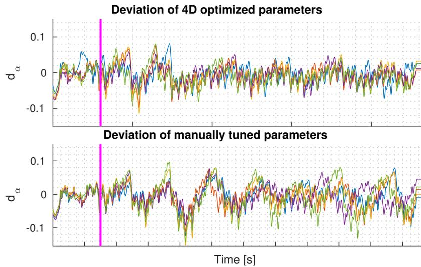
Figure 6.10: A comparison between manually tuned (top) and optimized (bottom) parameters during five longer real-world experiments, where the robot was walking 20 seconds instead of 10. Each curve shows the development of the Fused Angle deviation over the 25 seconds of the experiment. The vertical magenta line indicates the time at which the robot starts walking forward.
