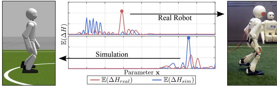
Figure 1.1: The proposed algorithm will trade off simulations with real experiments by maximizing relative Entropy.
