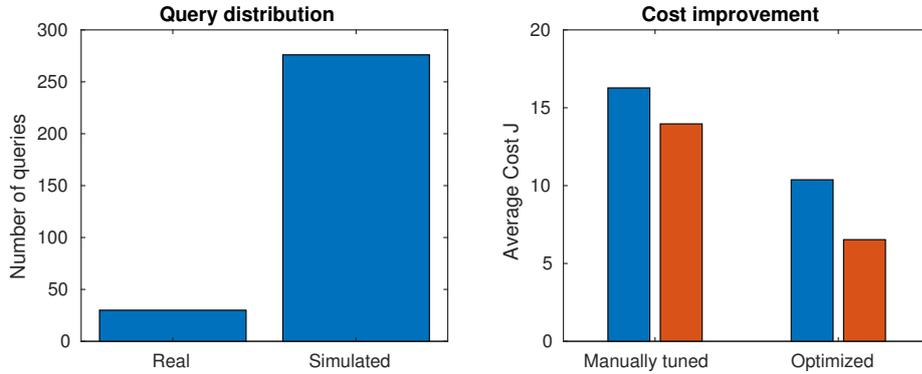
Figure 6.6: (left) 4D Optimization only using 30 real experiments (9.8% of total evaluations) thanks to the information gained through simulations. (right) The average sagittal cost of 15 evaluation is displayed, with (red) and without (blue) the penalty function. The algorithm chose larger parameters than previously, which were performing significantly better.
