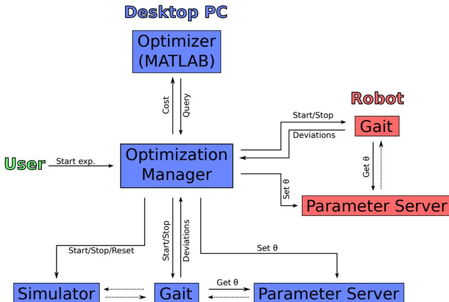
Figure 6.2: The used software architecture. The graph depicts the most important ROS nodes and the communication between them. The blue boxes indicate processes on the Desktop PC and the red boxes on the robot respectively.
