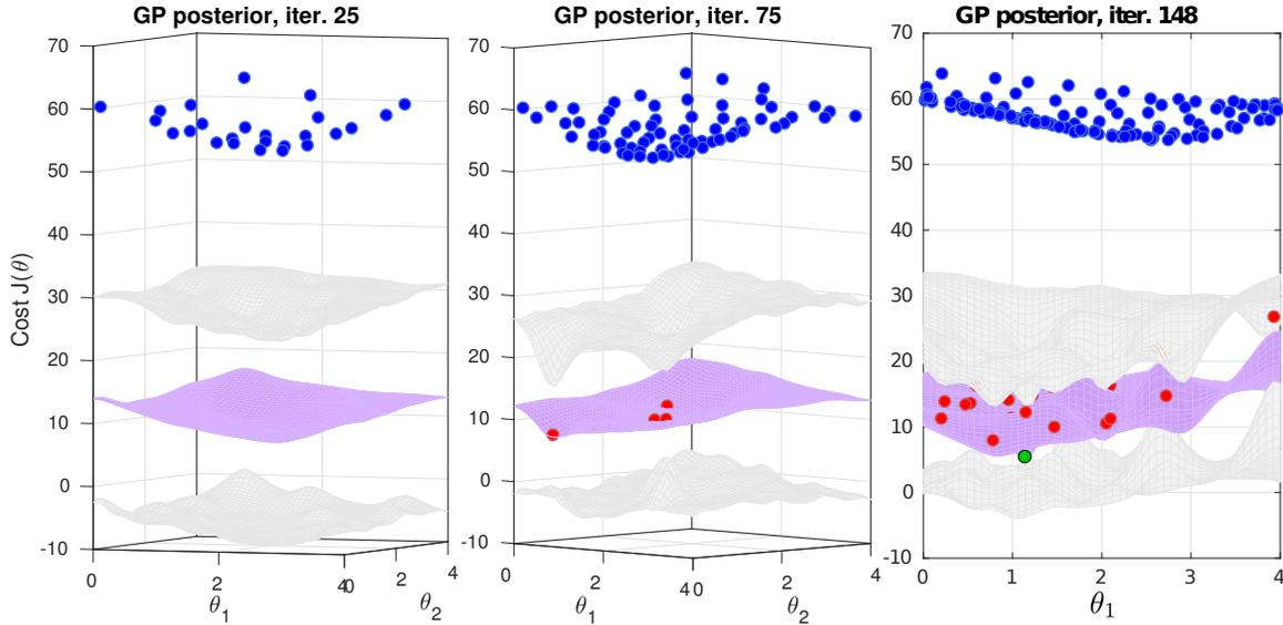
Figure 6.3: Visualization of the Gaussian Process after the 2D optimization of the ArmAngleY parameters. Real-world evaluations are shown red, whereas simulations are blue. The purple mesh resembles the posterior mean, the gray mesh shows the covariance and the green dot resembles the current minimum estimate. Due to the simulator error, simulations result in a higher cost. This transformation is learned by the GP to efficiently use simulator data in the learning process.
