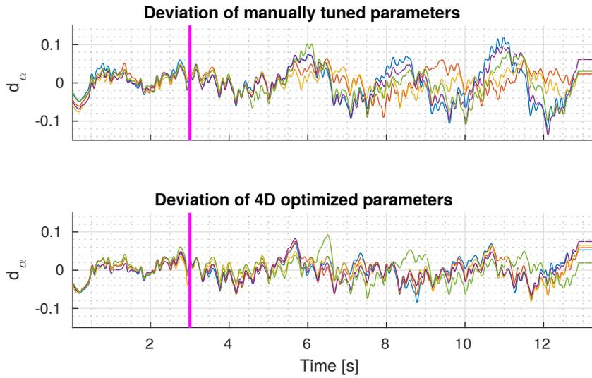
Figure 6.7: A comparison between manually tuned (top) and optimized (bottom) parameters during five real-world experiments. Each curve shows the development of the Fused Angle deviation over time in an experiment. The vertical magenta line indicates the time at which the robot starts walking forward.
