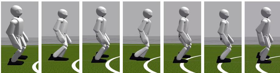
Figure 6.1: The igus<sup>®</sup> Humanoid Open Platform walking in simulation. The shown gait uses parameters resulting from a simulation-only optimization terminated by the KLD-threshold criterion.
