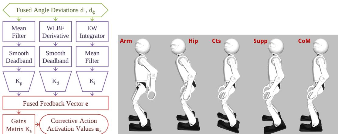
Figure 3.1: The feedback pipeline restricted to the used mechanisms (left) and a visualization of the Fused Feedback corrective actions in sagittal direction (right). **Note:** Adapted from [3].
