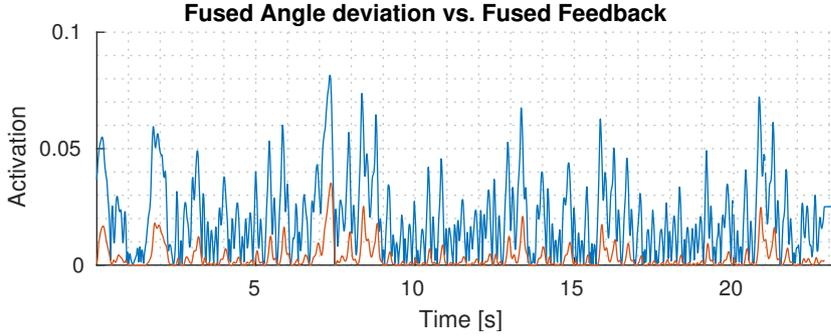
Figure 5.1: This figure displays the difference between the absolute Fused Angle deviations  $\|d_\alpha\|_1$  (blue) and the absolute proportional Fused Feedback  $\|e_{P,\alpha}\|_1$  (red). Due to the dead-band and mean filter, which are applied to the Fused Angle deviations to yield the Feedback values, the Fused Feedback signal is smoother and low amplitudes get rejected.
