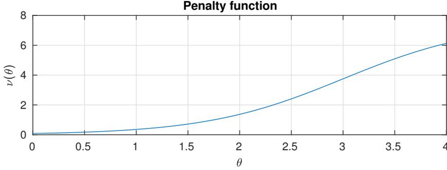
Figure 5.2:  $\nu(\boldsymbol{\theta})$  uses the logistic function to create a smooth penalty function against parameters of large magnitude. Here, we use  $\boldsymbol{\theta}_{max} = 4$ ,  $s = 7.5$ ,  $\lambda = 0.75$  and  $\gamma = 6$ .
