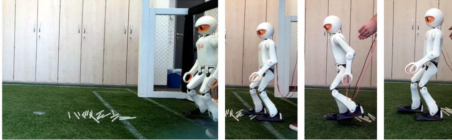
Figure 6.11: The setup of the disturbance test is displayed, where the robot has to walk over small obstacles. It is possible to see, that the disturbance destabilizes the robot temporarily.
