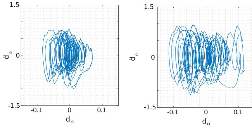
Figure 6.8: The deviation of a single pair of parameter is displayed as a phase plot (comp. Fig. 6.7). The X axis denotes the deviations, whereas at the Y axis its derivative is shown. It is possible to see, that the manually tuned parameters (right) lead to higher disturbances during straight walking compared to the optimized parameters (left).
