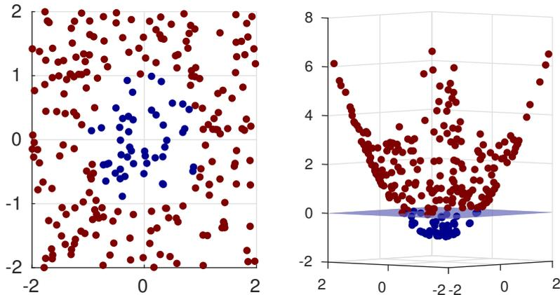
Figure 4.1: An example of linear separability in a higher dimensional feature space. The red and blue dots of the input data are not linearly separable in the input space (left), but if transformed into a higher dimensional feature space using a non-linear transformation  $\phi(x, y, z) = (x, y, x^2 + y^2 - 1)^T$  it becomes linearly separable (right).
