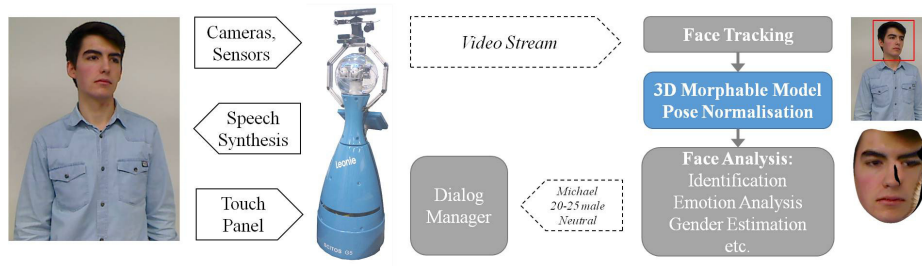
Fig. 7: Schematic overview of the framework for human-robot interaction on our SCITOS G5 platform. Our proposed landmark based 3D Morphable Model fitter acts as a pre-processing method for various face analysis tasks.
