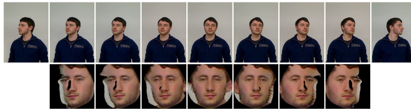
Fig. 8: Frames from a video of a subject turning from left profile to right profile view. The bottom row shows the pose-invariant isomap representations after fitting. Black regions depict self-occlusion/invisible parts of the face and thus cannot be drawn. On the two most extreme pose images, the initialisation with the face detector fails.
