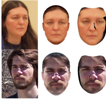
Fig. 4: From left to right: example images from PaSC (cropped to area of face for this figure) and their frontalised renderings from the commercial face modelling solution and our landmark-based fitter.
