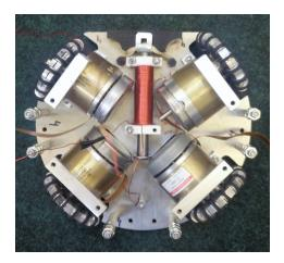
Fig. 5: Motors and kicker attached to chassis
