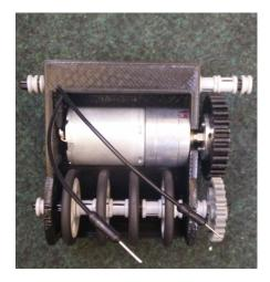
Fig. 6: Dribbler frame with motor and Lego roller
