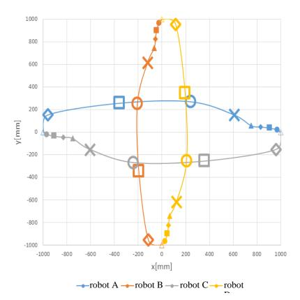
Fig. 14. Route of the 4 robots by avoidance simulation
