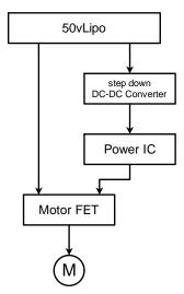
Fig. 4. Power line from Li-Po battery
