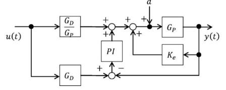
Fig. 6. Block diagram of control circuit
