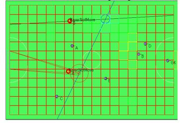
Fig. 13. Passing target and behavior of the receiver robot
