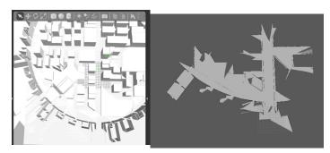
(a) Layout with displays in the model of Hall 1 (b) Output of hector\_SLAM
