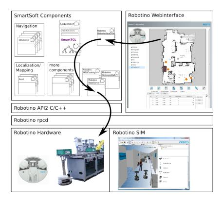
Fig. 2. The Robotino-SmartSoft integration.
