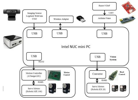
Fig. 3. Control architecture of HuroEvolutionTN robot.
