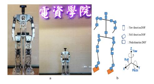
Fig. 1. HuroEvolutionTN. (a) Whole Body, (b) Structure design.
