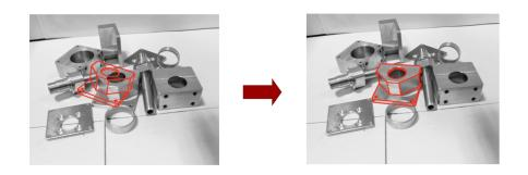
Fig. 6. An example of object registration using the  $D^2CO$  algorithm.
