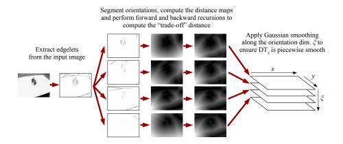
Fig. 5. DCD tensor computation pipeline.
