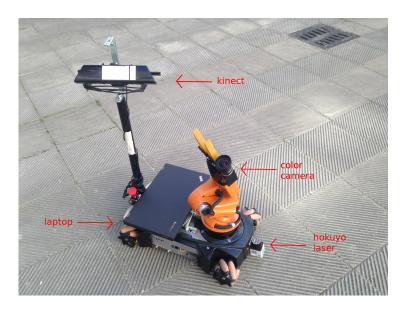
Fig. 1. The SPQR@Work robot  $\mathbf{F}$
