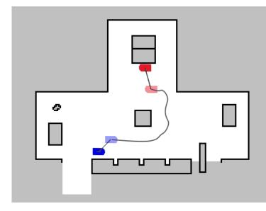
**Fig. 8.** An example of navigation path (dark gray). The curved portion of the entire path is computed by the primary navigation planner. Our potential fields based planner is used for approaching the final target (red) and for sliding away from obstacles at the beginning of the navigation task (blue).
