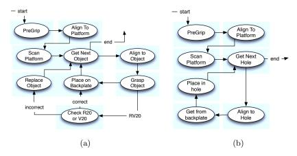
Fig. 5: (a) The simplified subtask-state-machine that is used for grasping objects at a service area. (b) The simplified subtask-state-machine that is used for dropping objects into the holes for PPT.
