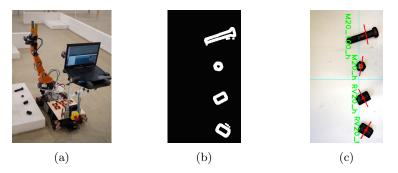
Fig. 4: (a) Pre-grip scan position. (b) Pre-processing of the image. (c) Detected objects, classification and grasp position of the closest object.
