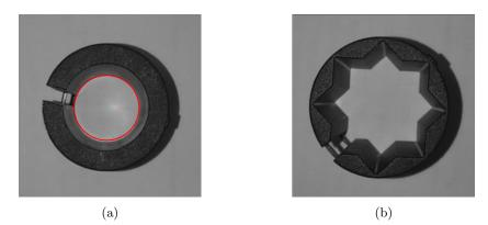
Fig. 3: (a) R20 object with detected circle. (b) V20 object with no detected circle.
