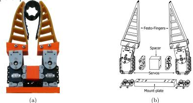
Fig. 2: Figure (a) illustrates the adaptation of the gripper to the round shape of the object. Figure (b) shows a drawing of the separate parts of the new designed gripper in more detail.
