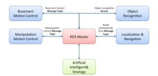
Fig. 3. Software framework based on ROS.
