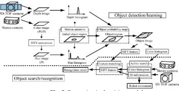
Fig. 2. Processing in the vision module
