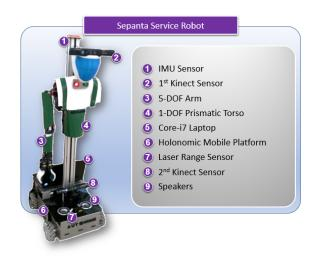
Fig. 1. Sepanta II equipment's description.
