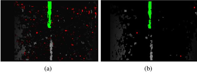
Figure 7: Disparity images of BM rectified using Chebychev calibration. False positives are colored red and the obstacle is overlaid with green. With the default settings shown in (a) the disparity map suffers from noisy estimates and speckles. (b) shows the resulting map after applying the speckle filter, resulting in less false positive measurements. The experiments showed that with increasing distance the number of speckles further increases.
