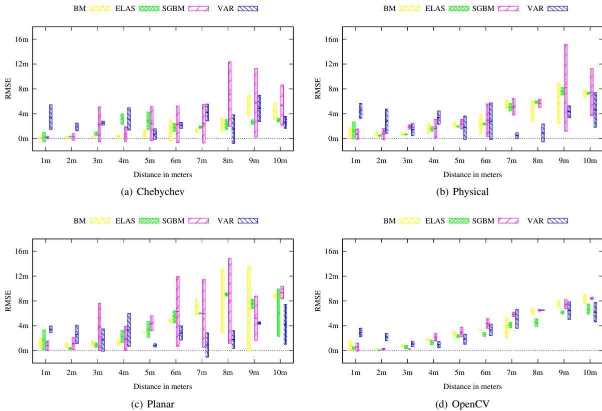
Figure 9: RMSE and corresponding variance of the depth measurements of the vertical cable under different calibrations. Error and variance are in general increasing with the distance.
