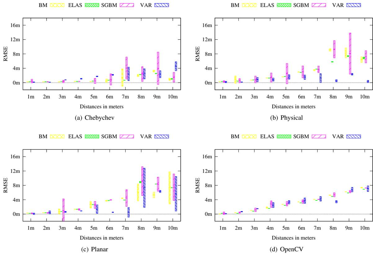
Figure 8: RMSE and corresponding variance of the depth measurements of the street light pole under different calibrations. Error and variance are in general increasing with the distance.
