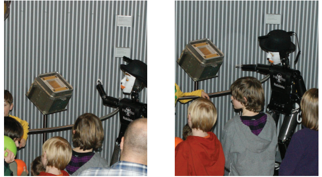
Fig. 5 Robotinho points at different object parts during its explanations to direct the audience's attention.
