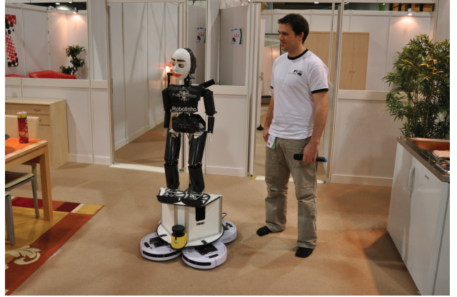
Fig. 3 Robotinho is placed on an omnidirectional wheeled base for fast and safe navigation. The total height of 160 cm simplifies face-to-face communication with adults.
