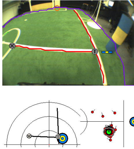
Fig. 1. Localization using line and corner features. The top-figure shows an image taken from the robot’s front camera. The purple line denotes the detected field boundary, red (green) lines show field lines (not) used for localization. Detected corners are marked as “X” or “T”. Bottom left: egocentric view with everything used for localization. Bottom right: resulting localization using the particle filter.
