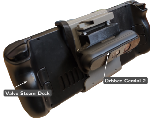
Fig. 2: Data-recording setup: We utilized an Orbbec Gemini 2 connected to a Valve Steam Deck supported by a guided data-recording procedure.
