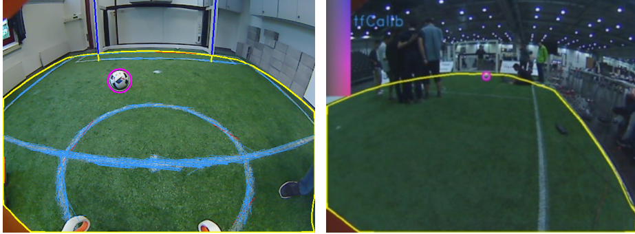
Fig. 5. Left: A captured image with ball (pink circle), field line (light blue lines), field boundary (yellow lines), and goal post (dark blue lines) detections. Right: Distant ball detection on RoboCup 2016 field.
