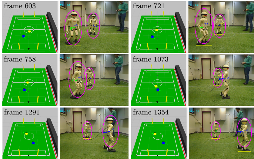
Fig. 5. Detection, tracking, and identification results obtained by our system.
