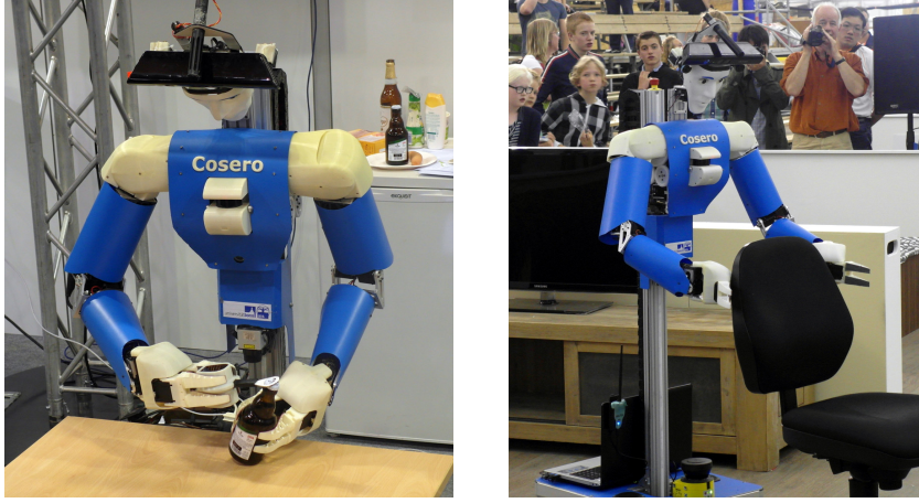
Fig. 1. The cognitive service robot Cosero . Left: Cosero opens a bottle during the final of the RoboCup@Home German Open competition 2014 in Magdeburg. Right: Cosero pushes a chair to its location during the Demo Challenge of RoboCup 2013, Eindhoven.
