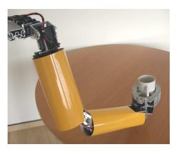
Fig. 3. 7 DOF human-scale anthropomorphic arm with 2 DOF gripper.
