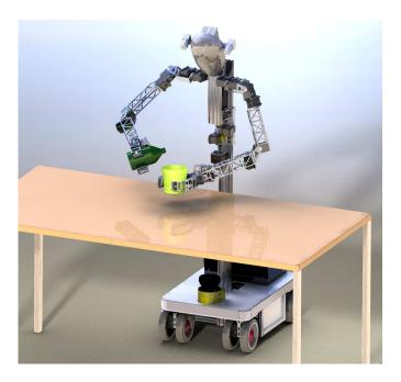
Fig. 7. Sketch of the anthropomorphic service robot Dynamaid with linear actuator in the trunk and second anthropomorphic arm for bimanual manipulation.
