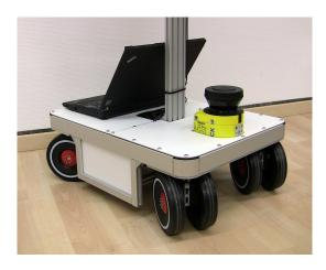
Fig. 2. Omnidirectional base with four individually steerable diff-drives.
