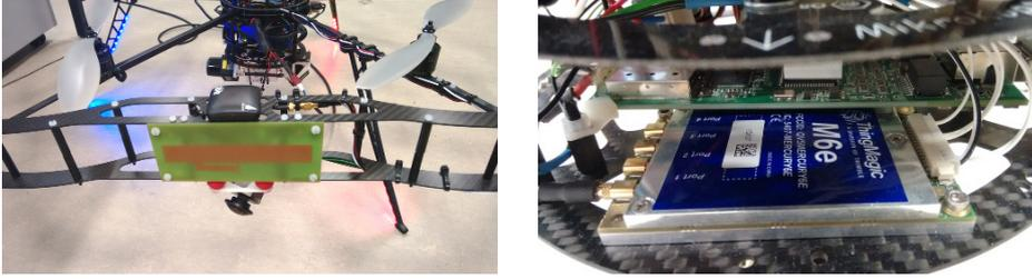
**Fig. 10.** RFID sensor. The MAV is equipped with a lightweight RFID antenna (left) and a small RFID reader module (right), connected to the onboard PC via USB. The RFID system is used to map positions of RFID tags in the allocentric map attached to shelves or inventory.
