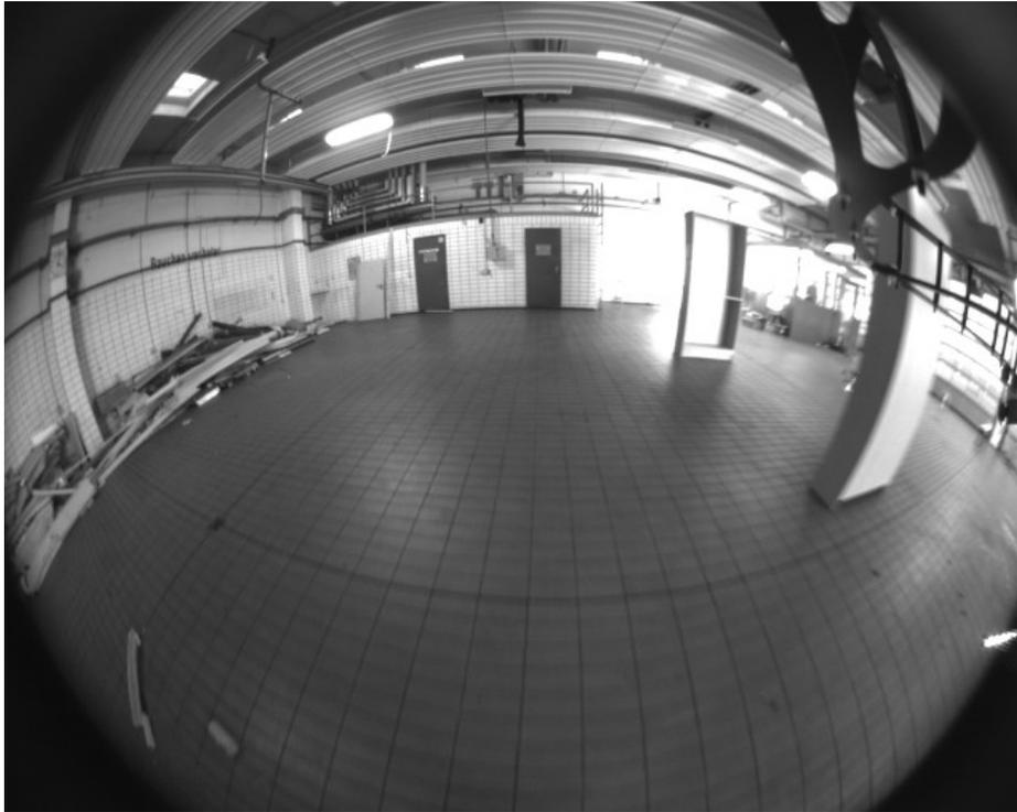
**Fig. 5.** Fisheye camera image of one of the onboard cameras. Due to the large FoV, the frame is slightly visible in the stereo configuration. We address this issue by either masking or by rectification which removes these artifacts.
