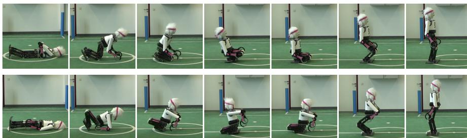
**Fig. 4.** Top row: Get-up motion from the prone posture. Bottom row: Get-up motion from the supine posture. In both motion sequences, the robot passively rocks back and forth on the foot edges from frames 3 to 5.
