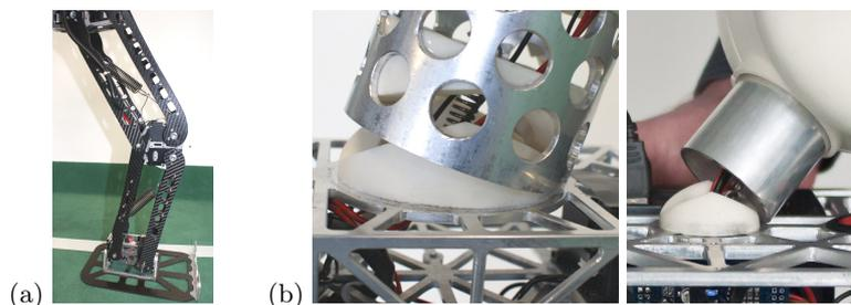
**Fig. 2.** Mechanical construction of Copedo: (a) leg with parallel kinematics; (b) spring-loaded overload protection in the hip and the neck joint.
