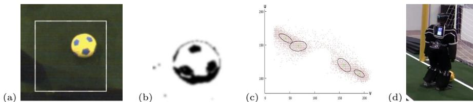
**Fig. 3.** Ball learning: (a) region of interest with unknown ball; (b) segmented pixels; (c) UV color histogram; (d) Dynaped completing the Dribbling Challenge.
