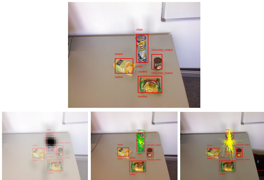
Fig. 2. Object recognition. Top: We recognize objects in RGB images and find location and size estimates. Bottom: Matched features vote for position in a 2D Hough space (left). From the features (middle, green dots) that consistently vote at a 2D location, we find a robust average of relative locations (middle, yellow dots) and principal directions (right, yellow lines).
