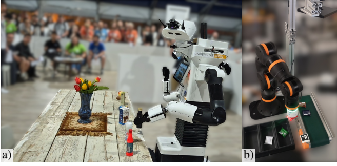
Fig. 4. Experimental robot platforms. (a) Team NimbRo's TIAGo++ robot at the RoboCup@Home 2024 finals in Eindhoven, grasping ingredients associated with a dinner recipe. (b) Industrial scenario where objects on a conveyor belt are detected from above, picked up, and placed in boxes.
