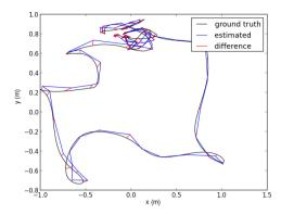
**Fig. 12:** Absolute trajectory error of the scan registration using the multiresolution map (blue) compared to ground-truth data from the MoCap system (black). Points of the trajectory are projected on the xy-plane.
