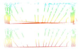
**Fig. 7:** Example of deskewing a 3D laser scan acquired in an indoor environment with flat ground from a side view. Sensor movement during scan acquisition yields distorted 3D scans (top). We deskew the scan based on the motion estimate (bottom).
