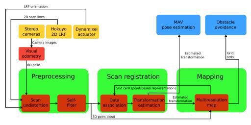
**Fig. 3:** An architectural overview of our system. The LRF measurements are processed in preprocessing steps described in Section 4. The resulting 3D point cloud is used to estimate the transformation between the current scan and the map as described in Section 5. Registered scans are stored in a local multiresolution map.
