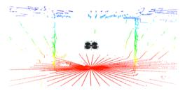
**Fig. 4:** A 3D scan of an outdoor environment acquired with our continuously rotating laser scanner. The colour of the points encodes the distance from the ground.
