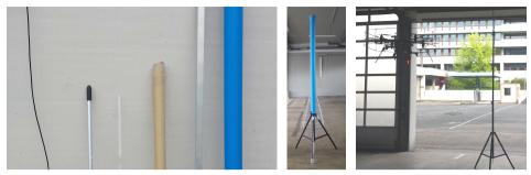
(a) Left: Different object types, from left to right: cable ( $\emptyset$ 0.75 cm), aluminium broomstick ( $\emptyset$ 2.7 cm), plexiglass tube ( $\emptyset$ 5 cm), cardboard tube ( $\emptyset$ 7.5 cm), rectangular metal rod ( $\emptyset$ 4 cm), blue plastic tube ( $\emptyset$ 11 cm). Middle and right: experiment setup with object holder, measuring tape and flying multicopter.
