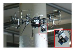
Fig. 1: The 3D laser scanner mounted on our MAV.
