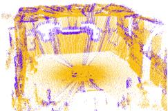
**Fig. 6:** Accumulated 3D scans of an indoor environment. Measurements from first echo (yellow) and the second echo (purple). In case of partial occlusions, e.g., by the MAV itself, multi-echo detection leads to an increase of distance measurements.
