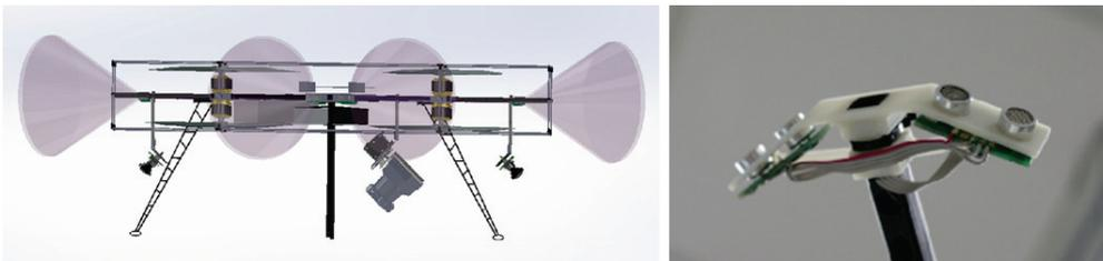
**Figure 9: Setup and mounting of the ultrasonic sensors. These sensors are used to reliably detect small obstacles in the close vicinity of the MAV.**
