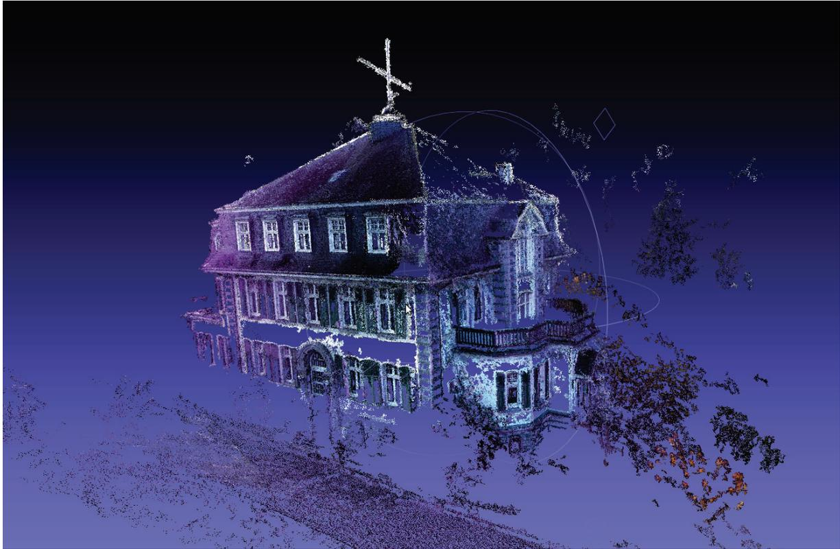
Figure 12: Georeferenced point cloud, extracted from images using a freely available software package for dense image matching (Furukawa, 2010).
