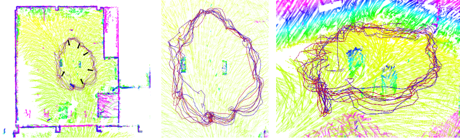
Fig. 15: We conducted indoor flight experiments in a 20 \times 16 \times 6 m hall. The trajectories show the laser-based localization estimates of 10 consecutive autonomous flights. From left to right: map top-view, closeup of the trajectories, perspective view. Observation poses are depicted by black arrows, the blue arrow shows the return pose. The map color encodes height.
