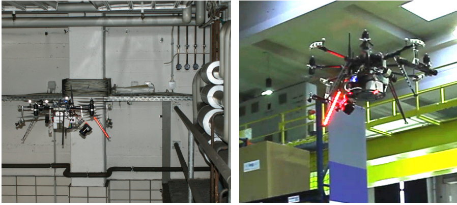
Fig. 1: Our MAV is equipped with eight co-axial rotors and a plurality of sensors, including a continuously rotating 3D laser scanner, two stereo camera pairs and eight ultrasonic sensors.
