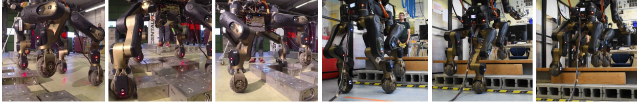
Figure 34: Complex locomotion tasks. Left: Traversing a step field. Right: Climbing stairs.
