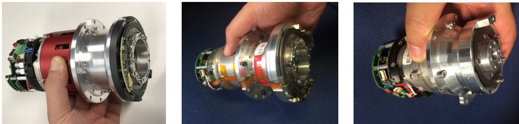
Figure 5: Manufactured actuation units of the identified classes (f.l.t.r.): Large, Medium, Small.
