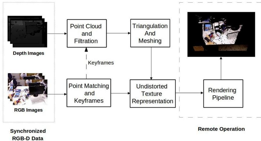
**Fig. 2.** Overview of our approach. The input to the system is depth image sequence (or point clouds) and synchronized RGB images. The output is 3D reconstruction of the environment which is efficient in computing, storage and capable to apply in real time.
