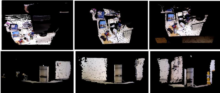
**Fig. 4.** Sample views generated from the approach used in this paper. (Top row) 3D reconstruction of three different views of the first sequence of the dataset. (Bottom row) 3D reconstruction of three different views of large cupboard of the dataset.
