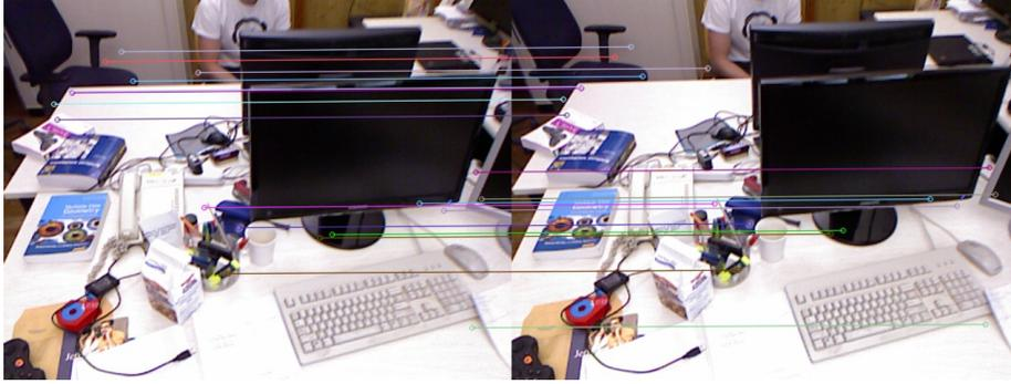
**Fig. 3.** SURF point matches between consecutive frames. Outliers are removed by applying a distance constraint on the vertical and horizontal shift between key points in consecutive frames. If the number of matched points  $N > 4$ , we consider these frames and calculate the transformation between two frames. Otherwise this frame is discarded and next frame in the sequence is incrementally considered for point matching.
