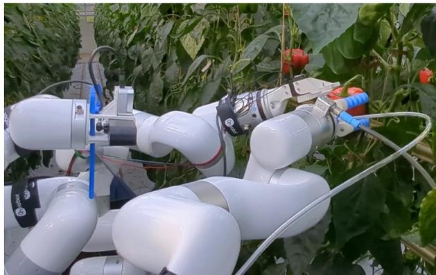
Fig. 1: HortiBot: A three-arm system with active perception and dual-arm manipulation for robotic horticulture. The right arm is used for grasping, the left arm performs cutting, and the central arm moves stereo cameras for mapping and online observation.
