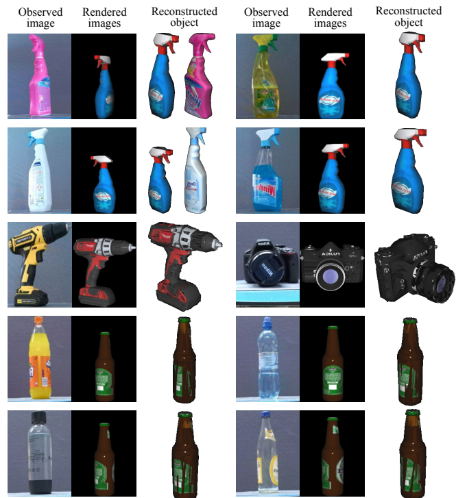
Fig. 11. Non-rigid registration on real pictures. The ground truth of two objects was available and is presented next to the reconstructed object. Hard objects to perceive as transparent bottles are successfully registered.
