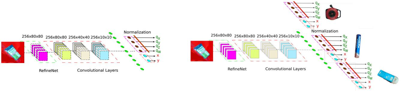
Fig. 4. Pose estimation network architectures. Left: Single-block output variant. Right: Multi-block output variant.
