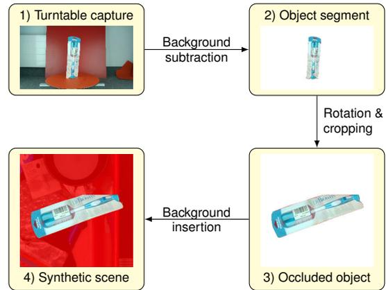
Fig. 2. Data acquisition & scene synthesis pipeline.
