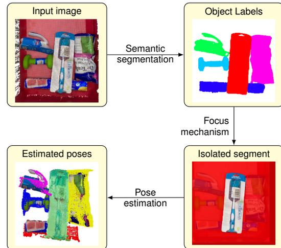
Fig. 1. The proposed 6D pose estimation pipeline for cluttered scenes.
