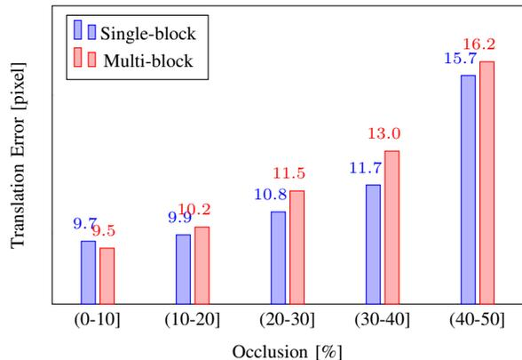
Fig. 7. Effect of occlusion on the translation error. The images in the validation set are grouped into different bins based on the percentage of pixels occluded.
