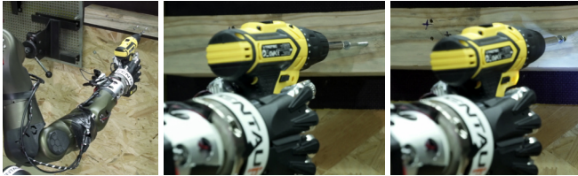
Fig. 18. Driving a screw into plywood. Left: Robot arm in front of the screw. Center/right: Detail on fine alignment and screwing.
