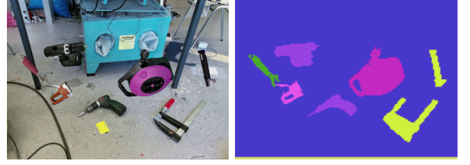
Fig. 5. Scene synthesis. Synthetic training scene generated by inserting new objects into the scene. The right image shows the resulting color image, the left one shows synthetic ground truth for training the segmentation model.
