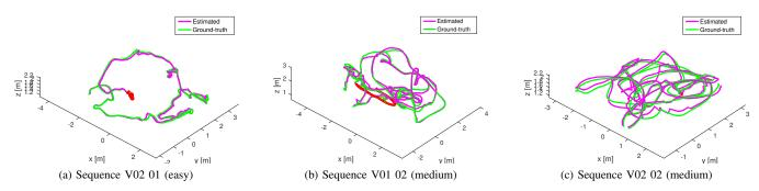
Fig. 3: Comparison of several trajectories from our approach with the given ground truth.
