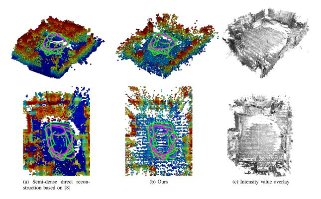
Fig. 4: Result for our first dataset showing the occupancy grid map by a semi-dense direct method (a) and the proposed feature-based method (b). The color encodes the height over the ground plane. The green curve denotes the Vicon ground truth, the magenta curve the estimated trajectory. Figure (c) shows the reconstruction from (a) overlaid with intensity values.
