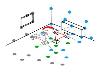
Fig. 1: The problem at hand: A (flying) robot equipped with multiple cameras traverses a scene orienting itself at distinct feature points that are tracked over time and between cameras. Observing points in multiple directions facilitates selflocalization and motion estimation during complex movements. The bottom camera can track this turning manoeuvre while the stereo camera cannot.
